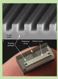
Reflective cell for cesium atomic micro-clock: (a) routing diffraction grating; and (b) packaged cell.
