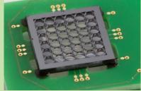
Array-type Mirau interferometer for swept-source optical coherent tomography: (bottom) matrix of Mirau interferometers; (top) 4-mm OCT scan of a sample made of scratched paint covered with varnish.
